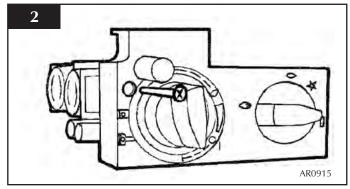
2.2 To release the right-hand side of the control cover insert the narrow blade screwdriver into the slot shown in diagram 3, lever it gently and pull from the right-hand side at the same time. The cover will now come off, there is a small cylindrical metal spacer inside the cover, this must be kept and replaced on the fixing screw during re-assembly.
